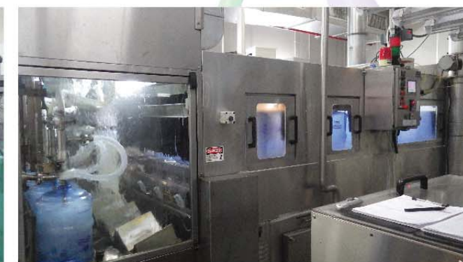
五加侖灌注機 Integrated Carboy washer / rinser / filler - improves the filling time to achieve a faster filling process
