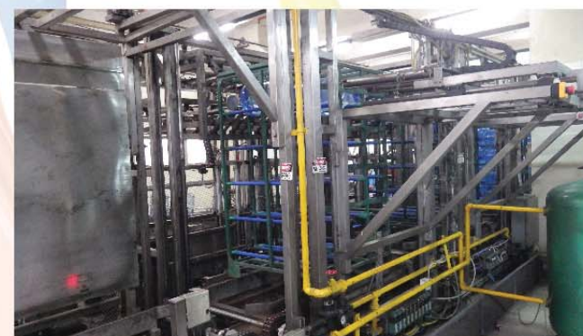
五加侖疊板機 Carboy Loader - new mechanical design improves the service life time and reduce downtime
