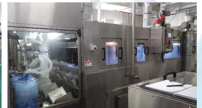
五加侖灌注機 Integrated Carboy washer / rinsers / fillers - improves the filling time to achieve a faster filling process
