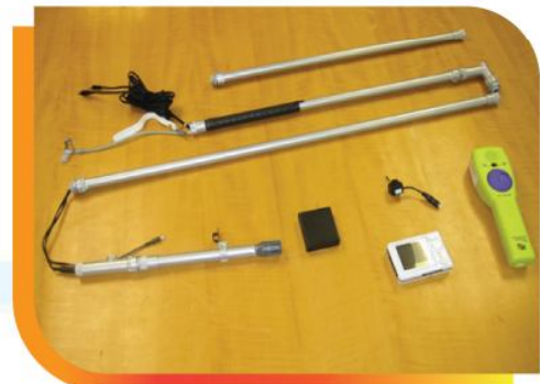
◎ 「視像寶」是附有視像功能，可改變長度及角度的測漏儀器 Advanced Gas Detector is retractable, expandable with varying angle positions incorporating a camera facility.
