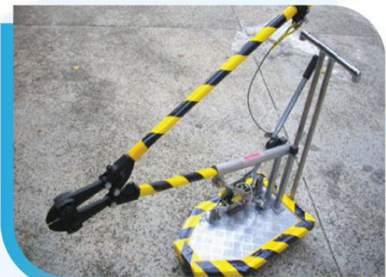
◎ 大力剪以槓桿原理設計 Apply lever mechanism in designing "Super Cutter"
