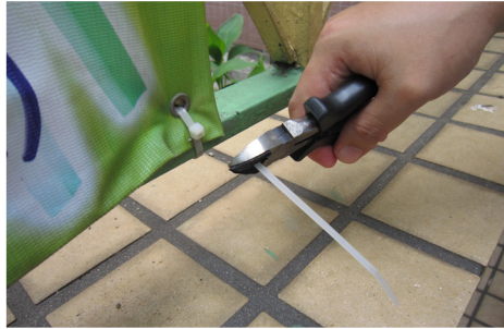
同時剪斷及抓緊索帶多餘部份 Cut and grab nylon strip ends simultaneously
